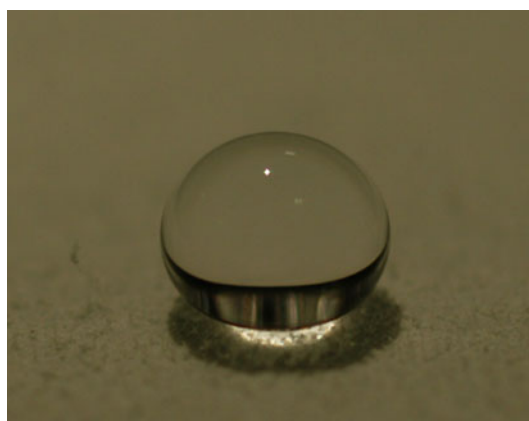
Fig. 1 A droplet of V_B = 30 \mu\text{L} fending off a hydrophobic surface
